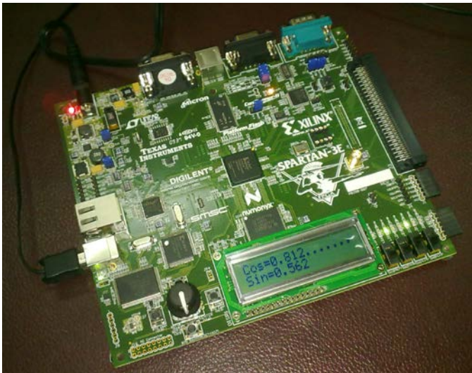
Fig. 5. CORDIC FPGA Implementation
